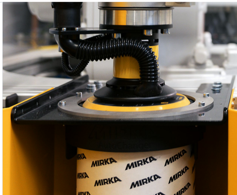
AIROS moving up, cylinder moving down (single puls).
