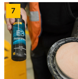
10 Polish with Deros RS 600, White Felt Polishing Pad + Polarshine E3
